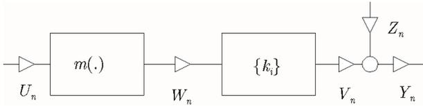
Fig. 1. Identified Hammerstein system.
